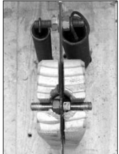
8. **Machete Roller Disk (F-2):** should be constructed from a  $\frac{1}{2}$ " thick laminated material like plywood or perhaps heavy duty plastic or fiberglass. You can glue two  $\frac{1}{4}$ " solid wood disk together positioned with the grain crossing. Do not use solid wood. There is a very heavy pounding force on this disk and it will easily shatter if made from solid wood.
