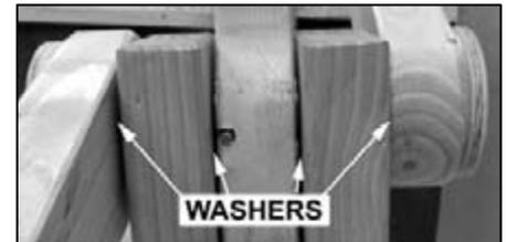
4. **Cam Axle (T-1):** As you go through the assembly process we suggest using the axle without drilling the holes for the axle pins that hold the cam and the handles. At the end of the assembly process you can then accurately locate the position for each pin and drill to fit the pins.
